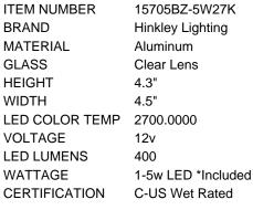
· Suitable for use in wet (interior direct splash and outdoor direct rain or sprinkler) locations as defined by NEC and CEC. Meets United States UL Underwriters Laboratories & CSA Canadian Standards Association Product Safety Standards
