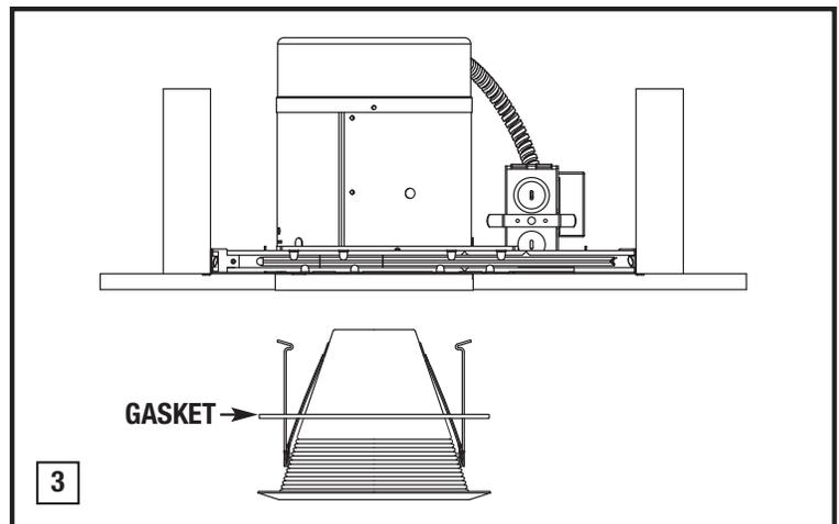
**REFLECTOR INSTALLATION (Figure 2):** Snap socket into hole provided in top of the trim or reflector. Install trim by pressing reflector around lip of trim and turn clockwise to lock into position.
